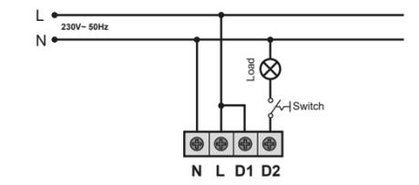
Installation with switch for permanent turning-on:
