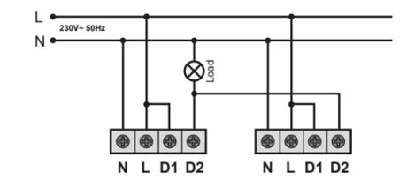
Installation with switch to enable or disable manually the motion detection:
