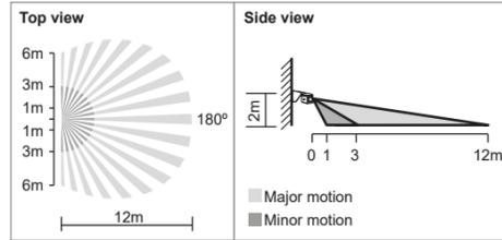
Walking direction: Pay attention to the walking direction at mount proceeding. The device is more sensitive to movement across the pattern than to movement directly towards detector. In the event that the motion is directly towards the detector, the coverage area will be reduced.
