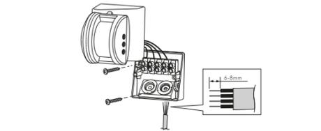
Fit the bottom cover on the wall firmly by two screws. Fix the detector head to the bottom cover and adjust the detector head to be in the right position.
