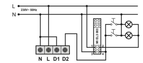
Installation with a timer (e.g.: MI PLA 002) and pushbuttons:
