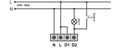
Staircase time switch (e.g.: MI EL3 003) controlled by one sensor:
