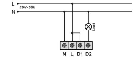
Two motion detections in parallel with one load:
